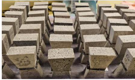
Fig. 2. Concrete specimens ready to be tested
